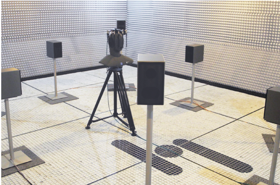
3PASS lab test setup in anechoic room with HMS II.3, MSA I and 8 loudspeakers
