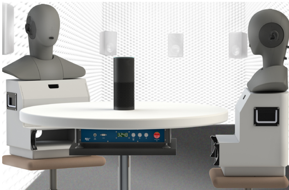
Measurement configuration with multiple talkers
